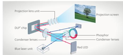
CASIO's unique optical engine combines a laser with an LED. It achieves high luminance by using light from a blue laser converted by the phosphor and the color wheel to complement the red light conventionally projected by red LEDs. The resulting light source realizes high brightness of 4000 lumens.
