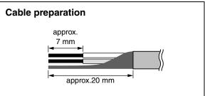
• To prepare the cable for attachment to a Euroblock connector, strip the wire as shown in the illustration using stranded wire to make connections. With a Euroblock connection, stranded wires may be prone to breakage because of metal fatigue due to the weight of the cable or due to vibration. Bundle the cables and the Euroblock tabs using the supplied cable ties (page 17). When rackmounting your equipment, use a lacing bar when possible to bundle and fasten the cables.
