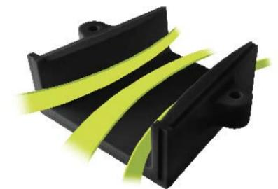
Internal faces of the port tube are profiled to ensure smooth air flow, reducing turbulence to increase low frequency efficiency and linearity at high power.
